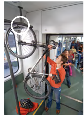
Place hook between spokes of front tire to hang bike upright.
