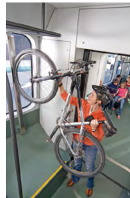
Metal "tire track" helps guide your front tire up to hook.
